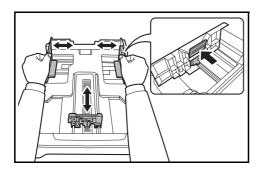
Adjust the position of the paper width guides located on the left and right sides of the cassette.
